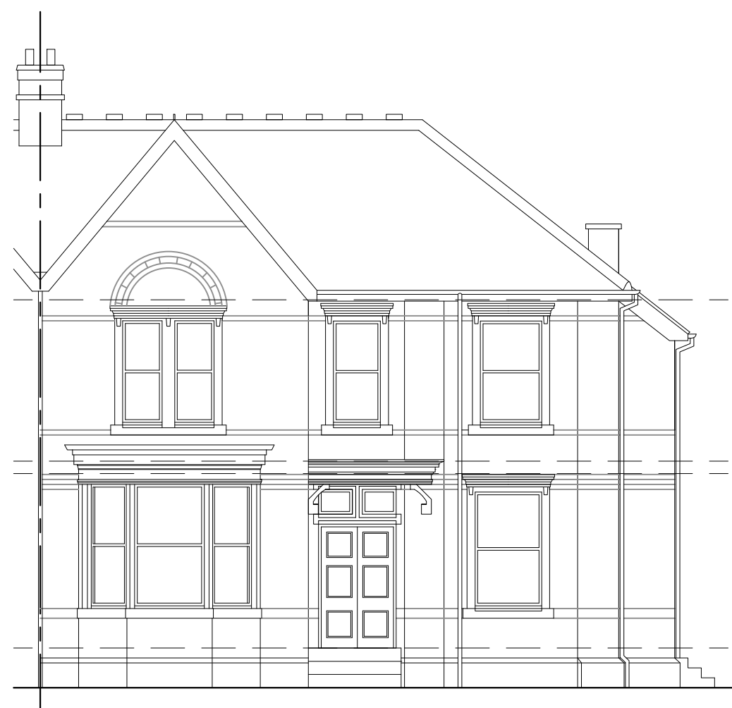
EXISTING FRONT ELEVATION SCALE 1:100
